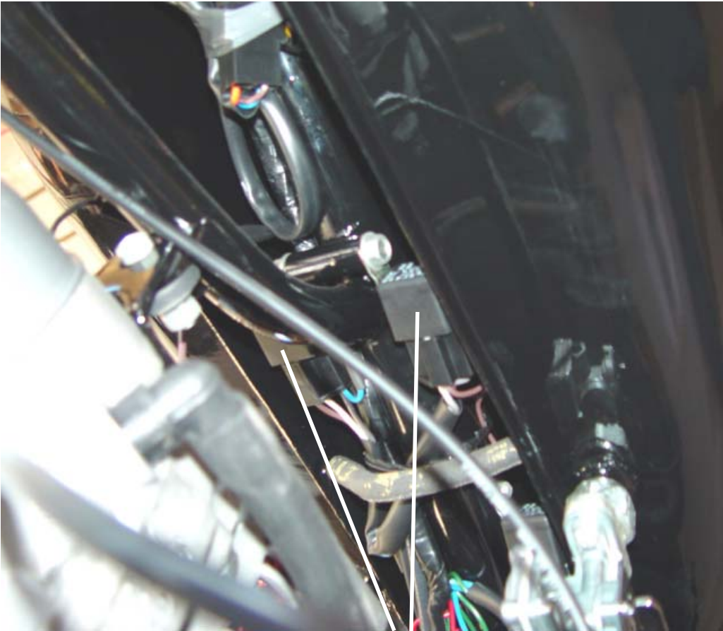
The fuse box is located under the front fork.
