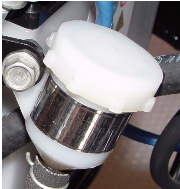
Rear Brake Hydraulic Reservoir
