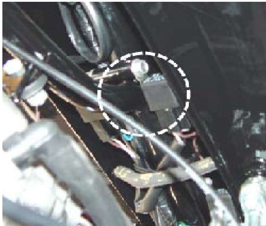
The headlight control relays # 1 & 2 are located underneath the fuel tank.
